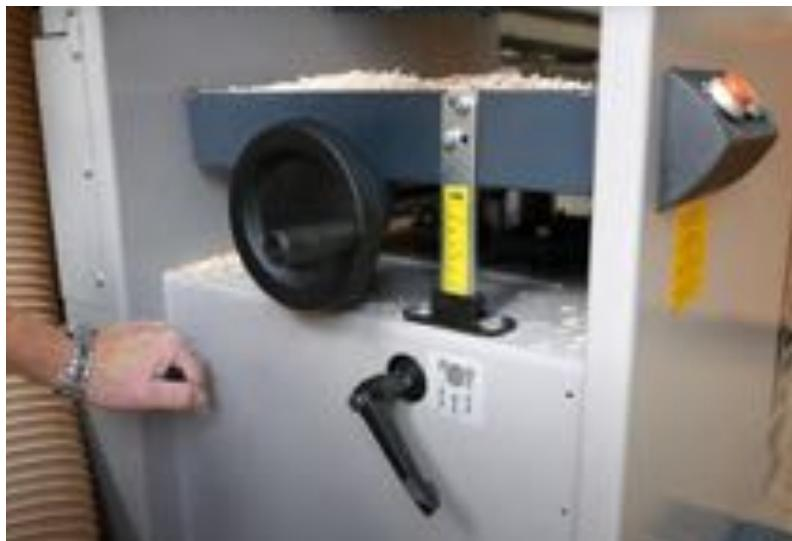
Planer-thicknesser in thicknessing mode. Note the feed-in engagement lever held by the operator's left hand.
