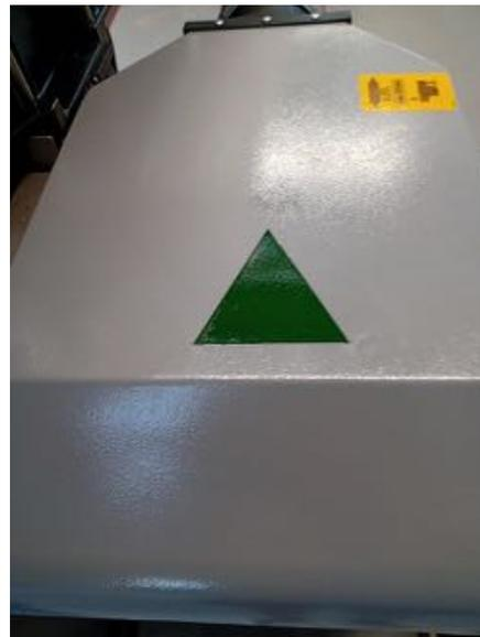
Hammer combination planer/thicknesser in thicknessing mode. Note green arrow for feed-in direction.
