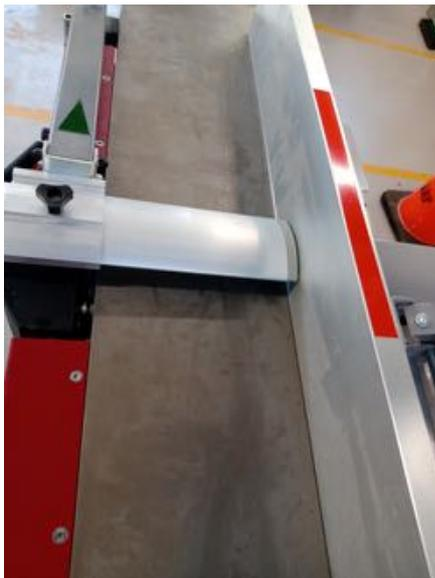
Hammer combination planer/thicknesser in planing mode. Note red zone on fence for location of fingers and green arrow for feed-in direction.
