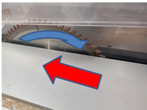
Note direction of feed (red arrow) and direction of rotation and teeth in blue.
