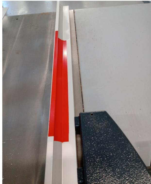
At a future stage the guards will be upgraded to incorporate flaps on both sides of the guards. In any case the guard must always be used and the height of the blade must be set no higher than material thickness plus 12-15 mm.
