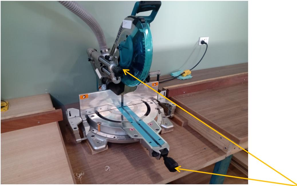
One of the two identical drop saws at LMCS, note the locking handles for the mitre and bevel adjustments.
