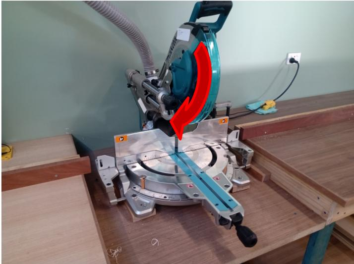
Figure 1 Direction of blade rotation, the same on all these types of saws
