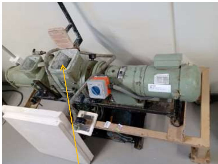
Figure 2 Pugmill, observe spinning worm inside the feed-in area, do not interfere
