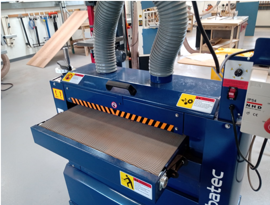
Picture 1 Drum sander power and feed speed controls on the right
